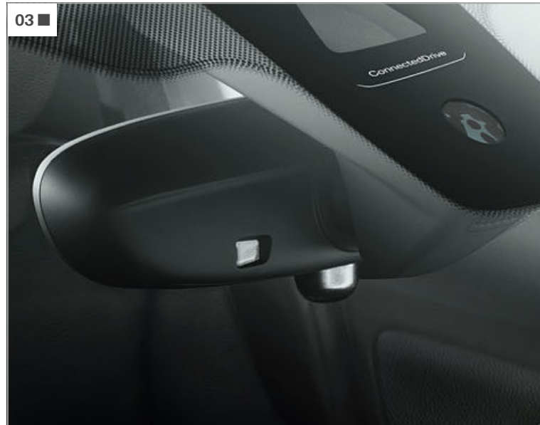
[ 03 ] The rain sensor including automatic headlight activation automatically switches on the windscreen wipers and the low-beam headlights.
