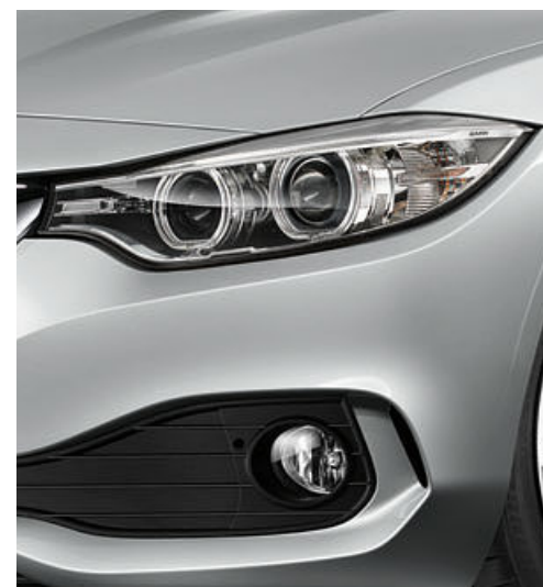
Xenon Headlights for low and high beam are included as standard and incorporate the headlight washing system, LED eyebrow and automatic headlight range control as well as parking lights and daytime driving lights via four illuminated corona light rings. Foglights in the front apron increase safety in bad visibility.
