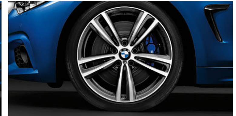
□ 2PL 19" M light alloy Double-spoke style 442 M with mixed run-flat tyres, 8J x 19, 225/40 R19 tyres front and 8.5J x 19, 255/35 R19 tyres rear.
